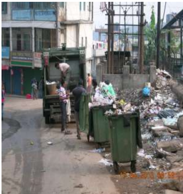
Loading & segregation in compactor
